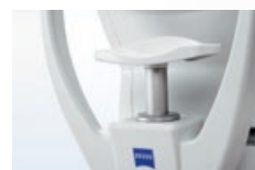
The motorized chinrest lets you quickly and comfortably position the patient
